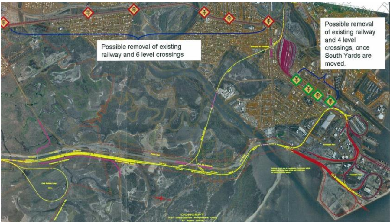
Figure 5.12 Alternative Alignment to allow the removal of Jetty Branch and section North Coast Line
