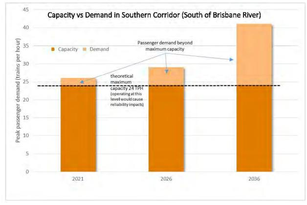
Figure 3.17: Rail Demand in Brisbane's South: Corridor Versus Available Capacity in the Morning One-Hour Peak<sup>36 37</sup>
