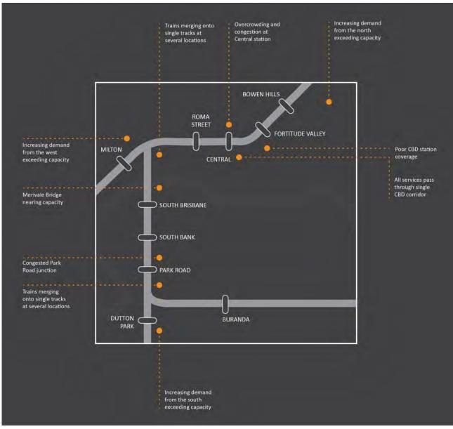
Figure 3.9: Existing Inner-City Rail Network Constraints<sup>26</sup>
