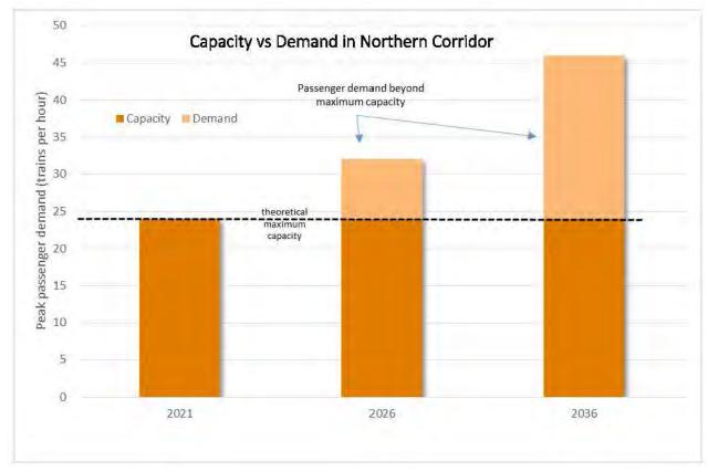
Figure 3.18: Rail Demand in Brisbane's North: Corridor Versus Available Capacity in the Morning One-Hour Peak<sup>38</sup>
